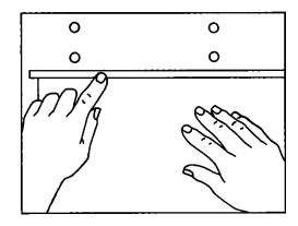
Flip the decal over the hinge and partially remove some liner, beginning at the hinge. Do not remove all liner to prevent presticking.
