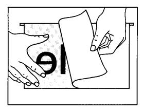
Without touching the adhesive of the graphic, apply it to the surface with a hard plastic squeegee with overlapping strokes. Proceed with application from the hinge to the other end of the decal.
