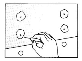
Push as much air out as possible and heat the film around each individual rivet with a hairdryer until the film softens. (Do not overheat !!). Push the film down with a squeegee or with your thumb for as close as possible to the rivet edge.
