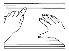
Application to this type of surface has to be done systematically: section by section should be covered with film as shown on the picture. Deviation from this application sequence may result in pleats that are impossible or difficult to get rid of.
