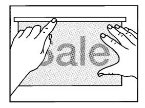
Flip the graphic back on the hinge and remove the liner partially, or if size allows entirely. Prevent the graphic to stick prior to application.
