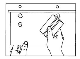
Once the entire decal has been applied and with the application tape still in place, punch with a needle some 4-5 holes around the rivet and proceed to apply the film with a squeegee. Once finished, remove all application tape.
