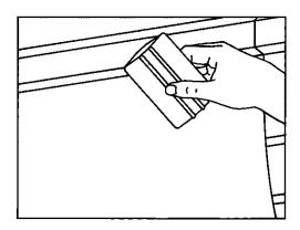
Try as much as possible to use the full width of the squeegee to press the film down over the entire surface area to be applied. Vertical sections to be applied by vertical squeegee strokes.
