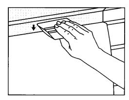
Make sure the film is applied well in the edges that border the individual sections. Remove application tape after some minutes and check and resqueegee the edges.
